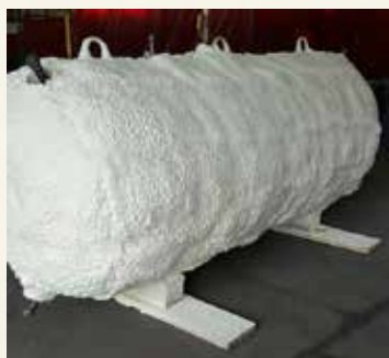
Closed, Repurposed Propane Tank With Spray Foam Insulation Applied
