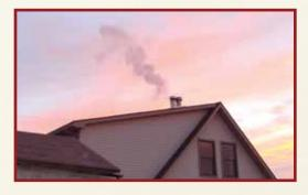
This is exhaust emitting from the **Wood Gun<sup>™</sup>** gasification boiler. What you see is not smoke but the moisture condensing due to cold temperature. (notice the vapor trail ends within a small distance)
