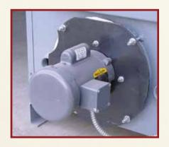
A high velocity, variable speed draft fan moves air through the wood allowing for easy cold start up. After the gasification process begins this air movement produces intense flames and very high temperatures in the gasification tunnel. In turn The air flows through the heat exchanger, cleaning it as it passes through.
