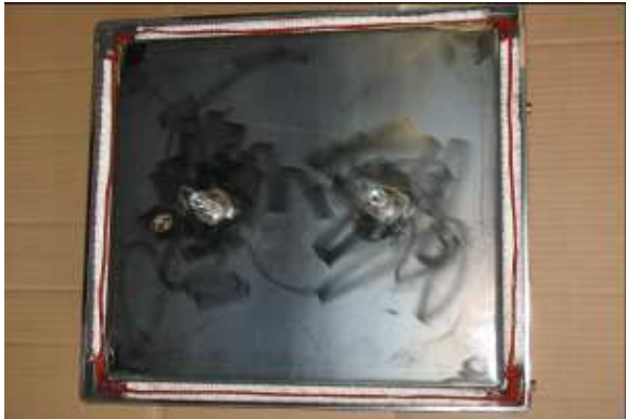
Load Door with Fiberglass Braid Tape and More High Temperature Silicone
