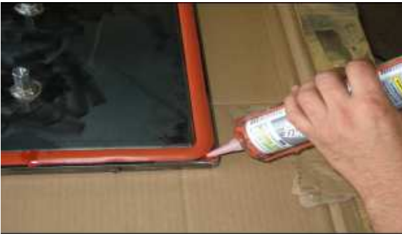
Reinforcing Corners with High Temperature Silicone
