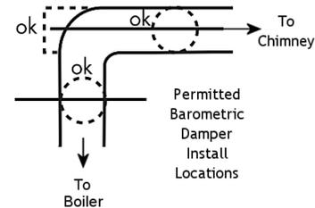
It is important to check the chimney draft when the seasons change to ensure draft settings are correct. Changes may be needed when transitioning from winter heating to summer heating (domestic water heating). The amount of draft will change from one season to the next. It is not uncommon to add a draft inducer in warmer seasons to maintain the recommended -.04 to -.07 inches of water column.
