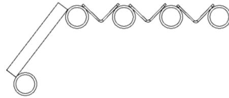
**Side View of Steel Angle Baffles in Position**
