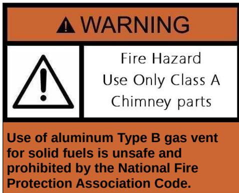
The boiler must be connected to a Class A chimney. Use of aluminum Type B gas vent for solid fuels is unsafe and prohibited by the National Fire Protection Association Code. There are three types of Class A chimneys:
