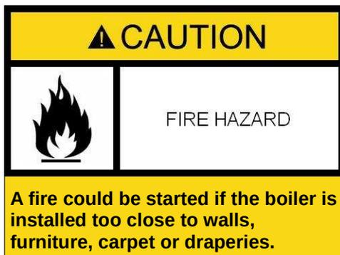
The boiler must be installed in an area dedicated to the boiler and its related equipment. This area must be partitioned or separated from any living area of a residence. The room must have a constant fresh air supply to assure proper combustion of the fuel as well as ventilation of any by-products of combustion.
