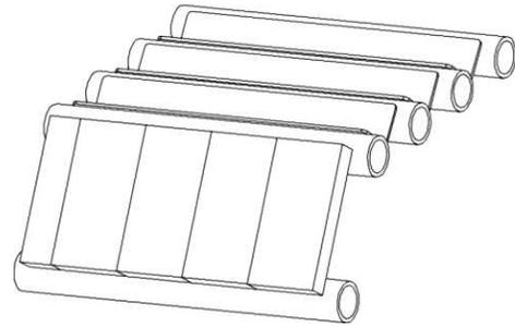
**Angled View of Steel Baffles Over Water Tubes**
