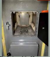
The firebox of the SE110 can accommodate wood sizes ranging from unsplit logs to full rounds and up to 26" long.
