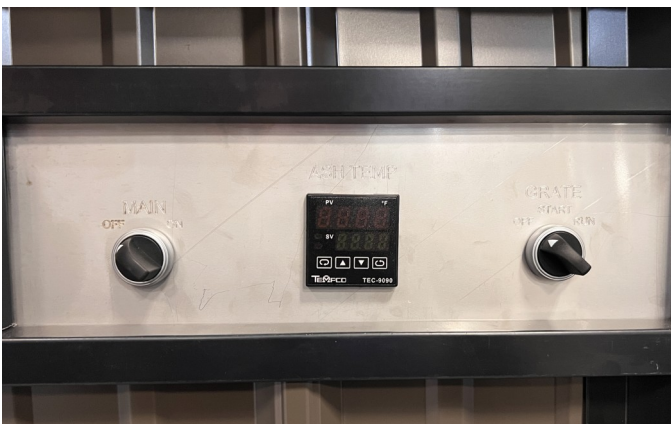
Switches and Digital Controller for Thermal Ash Control
