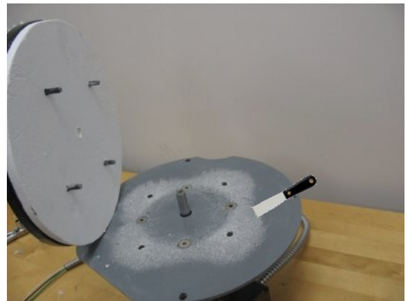
Separate Heat Shield from Motor Mount Plate
