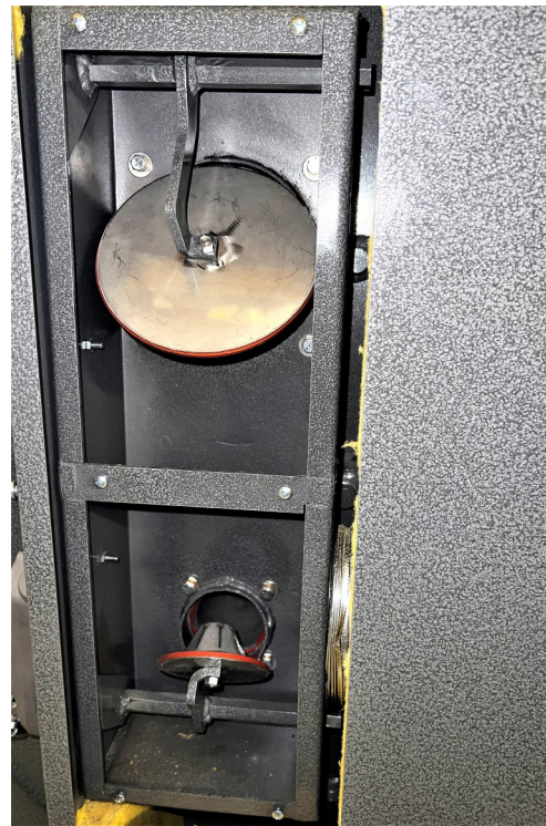
Air Valve Disk in Open Positioning
