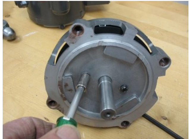
Loosening Screws Securing Bearing to End Shield
