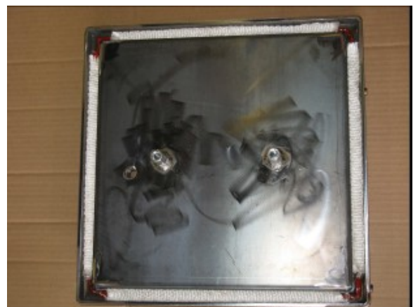
Load Door with Fiberglass Braid Tape
