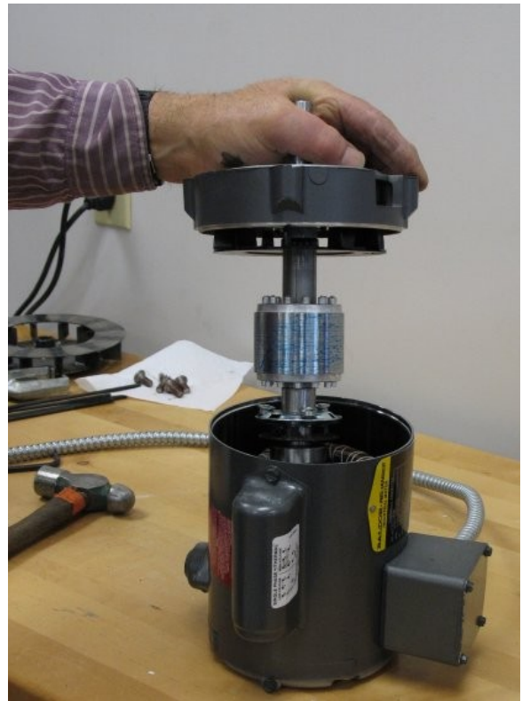
Lifting the End Shield with Armature
