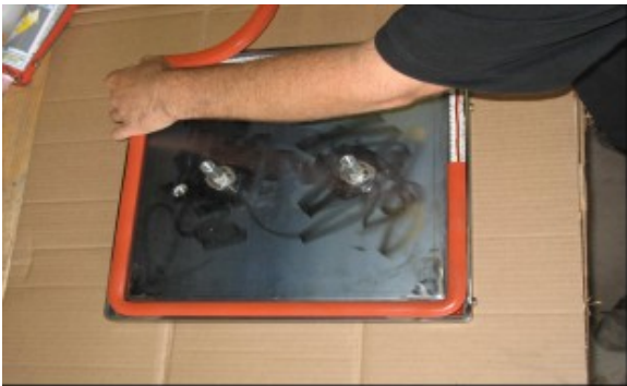
Adding Preformed Silicone Bead to Door
