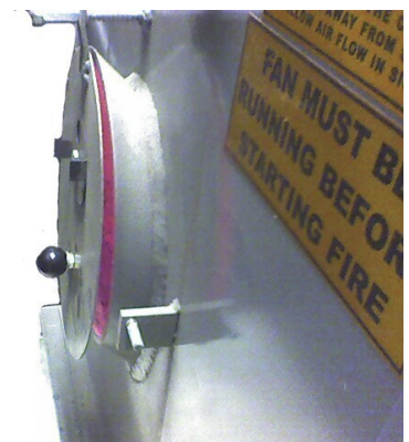
Sight Tube Flap in Open Position (Sight tube cover removed)
