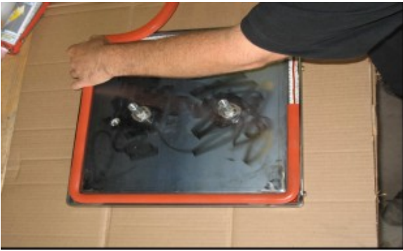
Adding Preformed Silicone Bead to Door
