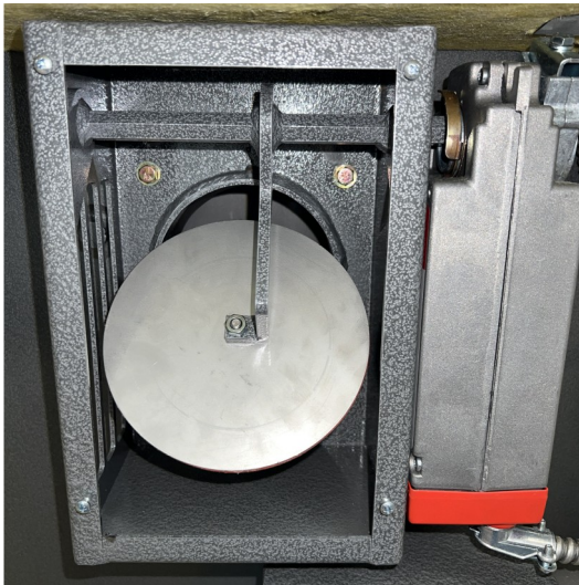
PRIMARY Air Valve Disk in Open Positioning
