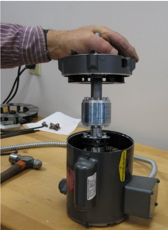
Lifting the End Shield with Armature
