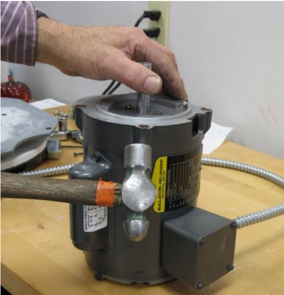
Loosening Motor End Shield from Motor
