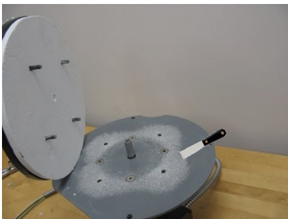
Separate Heat Shield from Motor Mount Plate
