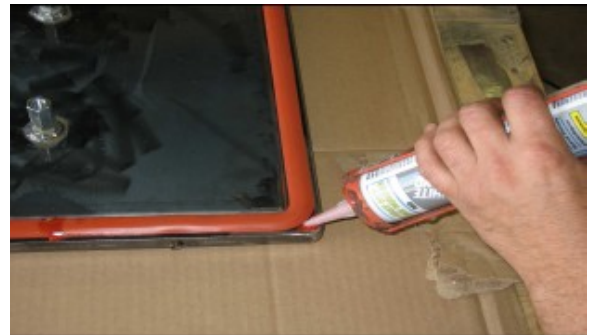
Reinforcing Corners with High Temperature Silicone
