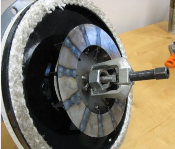
Jaw Puller at the Ready
