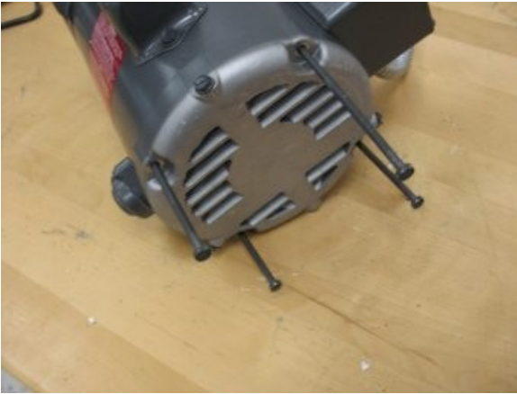
Motor Frame Assembly Bolts
