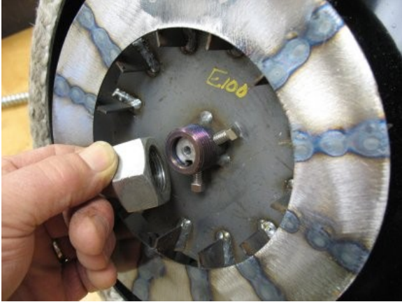
One Inch Nut for Pulling Fan
