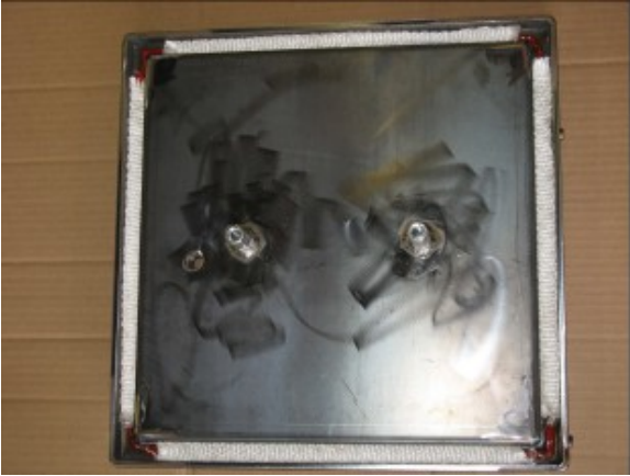
Load Door with Fiberglass Braid Tape
