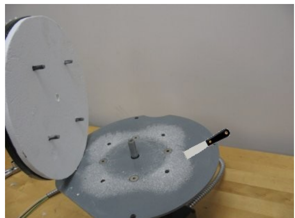
Separate Heat Shield from Motor Mount Plate
