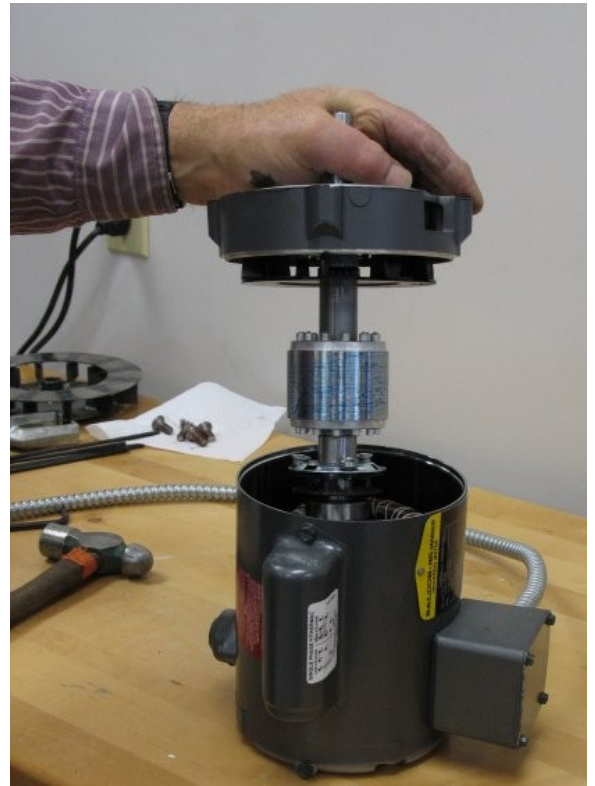
Lifting the End Shield with Armature
