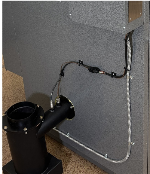
O2 Sensor and Thermocouple wires
