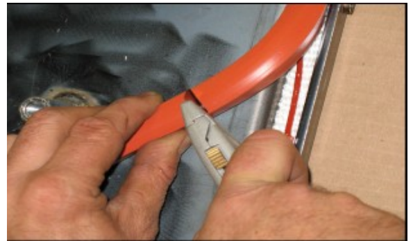
Trimming Preformed Silicone Bead
