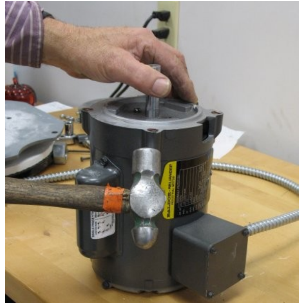
Loosening Motor End Shield from Motor
