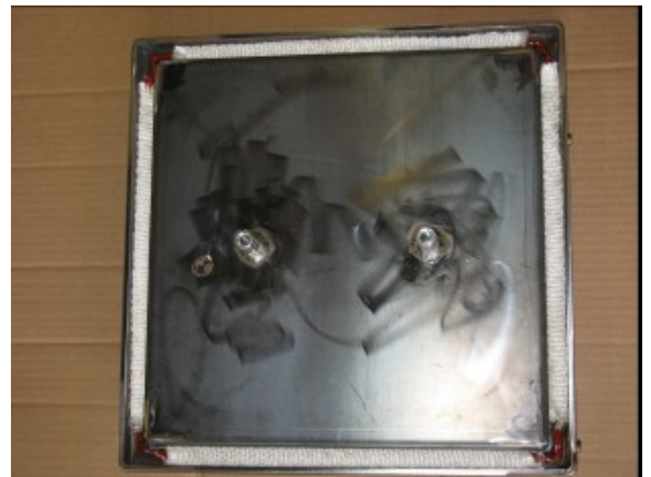
Load Door with Fiberglass Braid Tape
