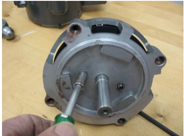
Loosening Screws Securing Bearing to End Shield
