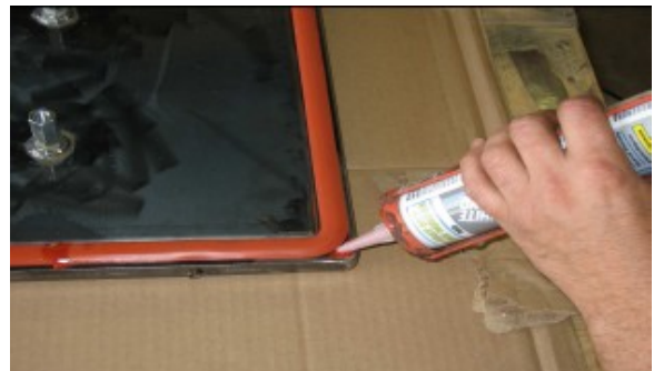
Reinforcing Corners with High Temperature Silicone
