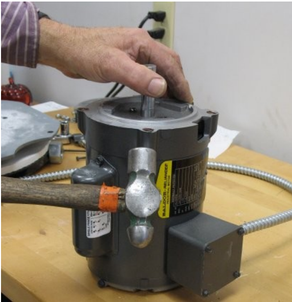
Loosening Motor End Shield from Motor
