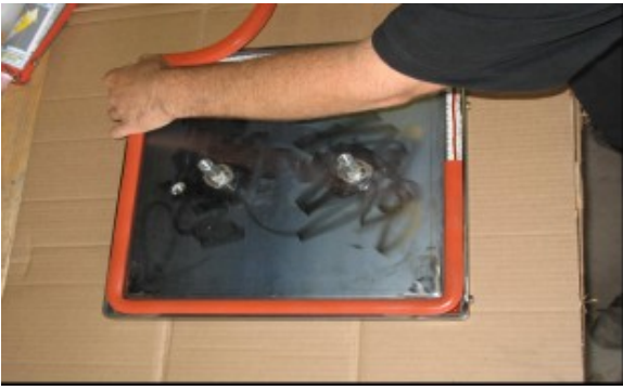
Adding Preformed Silicone Bead to Door
