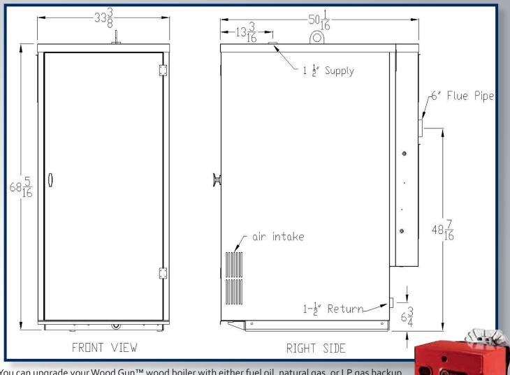
You can upgrade your Wood Gun™ wood boiler with either fuel oil, natural gas, or LP gas backup (non-UL version only). The Riello fuel oil burner will allow you the option of automatic backup. Upgrading your wood boiler enables you to save money by burning a renewable fuel source and the convenience of burning oil. The oil backup system is rated over 84% efficient. You can't go wrong with an efficiency rating that rivals top-of-the-line oil units.
